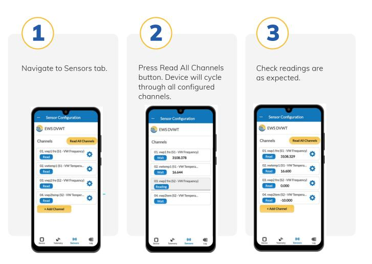
To change channel configuration or measurement interval – navigate into each channel and change as required.
