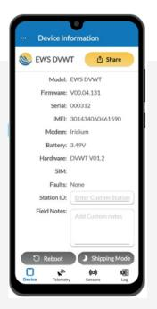
**Device tab** is where you can find all general Device information such as hardware version, firmware version, IMEI number, Devices internal battery voltage as well as custom station ID field and site notes. This is also where device reboot and enter shipping mode buttons are found.
