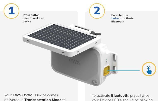
delivered in **Transportation Mode** to conserve battery life until installation. To wake up your Device, simply press button once. To activate **Bluetooth**, press twice your Device LED's should be blinking Blue and Green indicating it is ready to be paired with **EWS Lynx** mobile configuration App.
